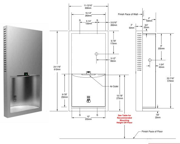
Rough Wall Opening 10-7/8" (277mm) wide 23" (585mm) high 4" (100mm) minimum recessed depth
